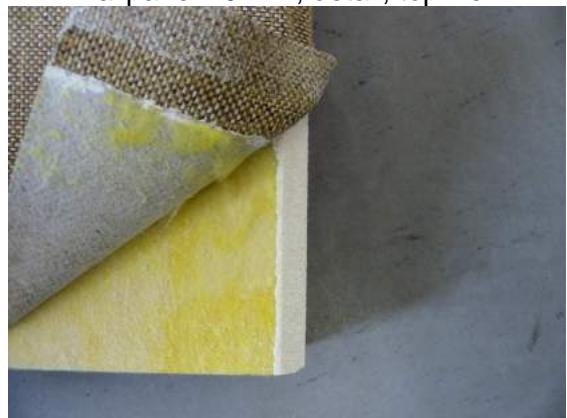
Wallpanel 40 mm, detail, top view
