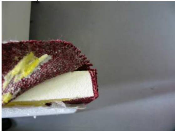
Wallpanel 20 mm, detail, side view
