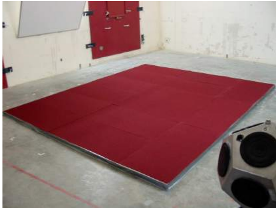
Wallpanel, thickness 20 mm, under test
