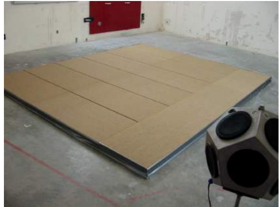
Wallpanel, thickness 40 mm, under test
